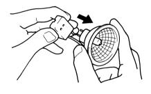
Remove the Projection Lamp from the Lamp Holder.
